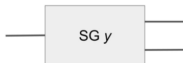
Figure 3.8. Simplified notation for an ordinary Stern-Gerlach device oriented along the y direction. The top beam corresponds to the positive y direction, and the bottom beam corresponds to the negative y direction.
