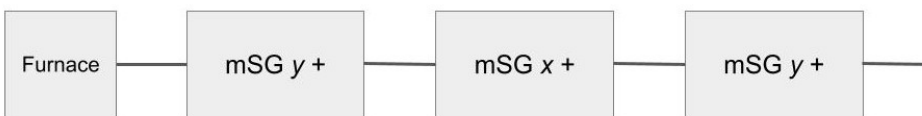
Figure 3.20. Chain of 3 devices yielding the amplitude \langle \uparrow y | \uparrow x \rangle \langle \uparrow x | \uparrow y \rangle .
