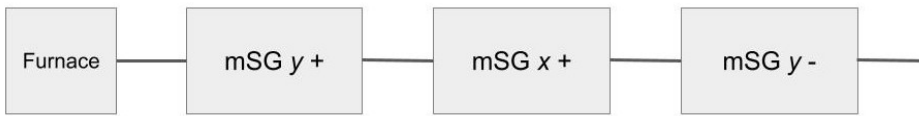
Figure 3.19. Chain of 3 devices yielding the amplitude \langle \downarrow y | \uparrow x \rangle \langle \uparrow x | \uparrow y \rangle .
