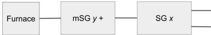
Figure 3.12. Measuring the spin in the x direction after having filtered in the y direction.
