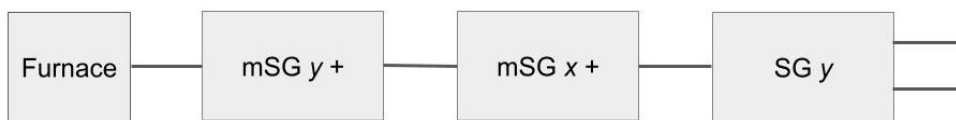
Figure 3.14. Three device experiment. Despite having filtered for the y+ direction, the end result is completely random.
